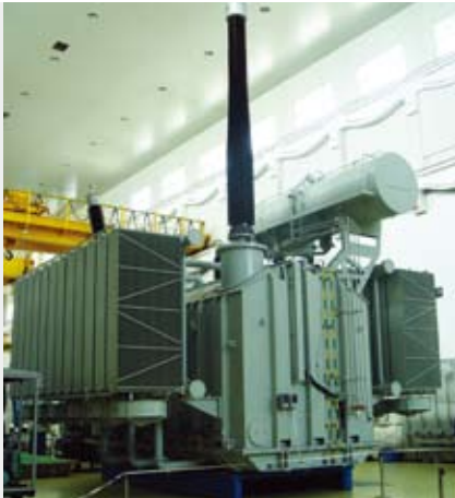
保变——四川崇州变电站扩建 ODFS – 334MVA/525KV Baoding Tianwei-Chongzhou, Sichuan province, transformer substation expansion ODFS 334MVA/525KV
