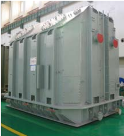
沈变——小湾电厂 DSP-260MVA/500KV Shenyang transformer-Xiaowan power plant DSP-260MVA/500KV
